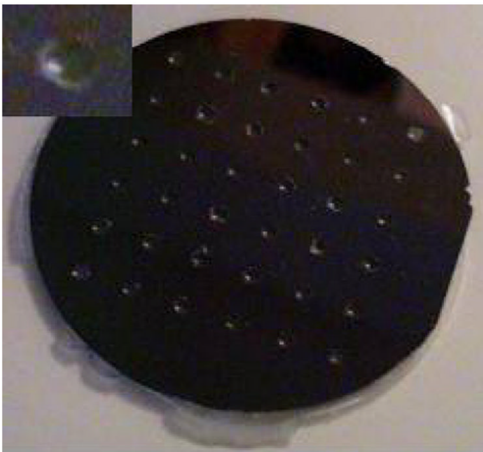
Fig. 20. Shaped wax mold on the silicon substrate [125].
