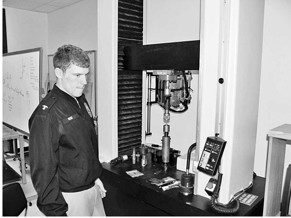
Figure 3. Midshipman conducting tensile testing of copper specimens in support of Electromagnetic Launcher (EML) program.
