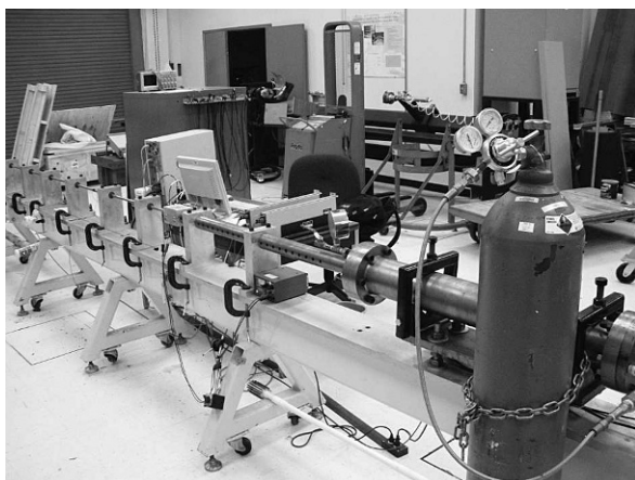
Figure 4. Split Hopkinson Pressure Bar (SHPB), with gas gun and gas source in right foreground and impact bar on left-hand side of the image.
