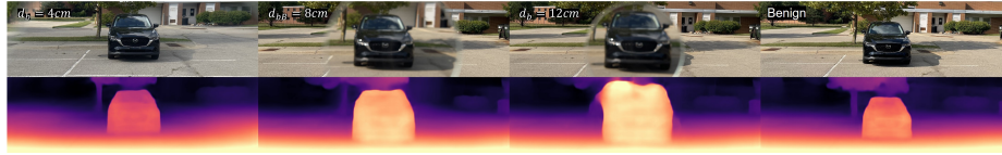
Fig. 9: The convex lens attack on an iPhone with d_{o1} = 9m , f = 50cm , and various d_b .
