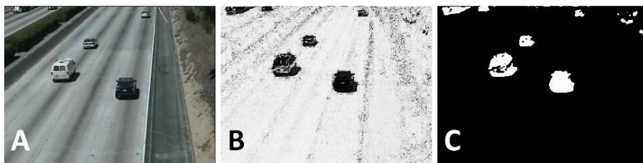
Figure 6.2: Results from a 500 frame sequence in which there is no training period without moving objects. A - input frame. B - probability map as calculated by Eq. (4.5), white means high probability to be in the background. C - Segmentation.
