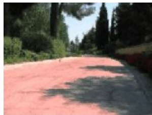
Figure 13: Shadows can cause mistakes in the road (marked in red) finding process.
