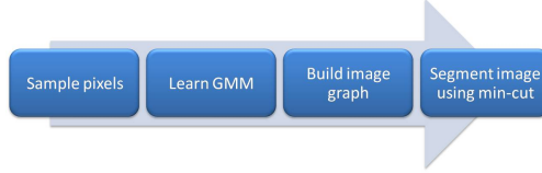
Figure 7: Vision system flow diagram. First we sample pixels to obtain a data set in which we can perform the learning process. Then we learn the parameters of two Gaussian Mixture Models using the data set. We use the GMMs to assign road and non road probabilities for each pixel. After that we build the image graph using the calculated probabilities, and finally we segment the image by cutting the graph.
