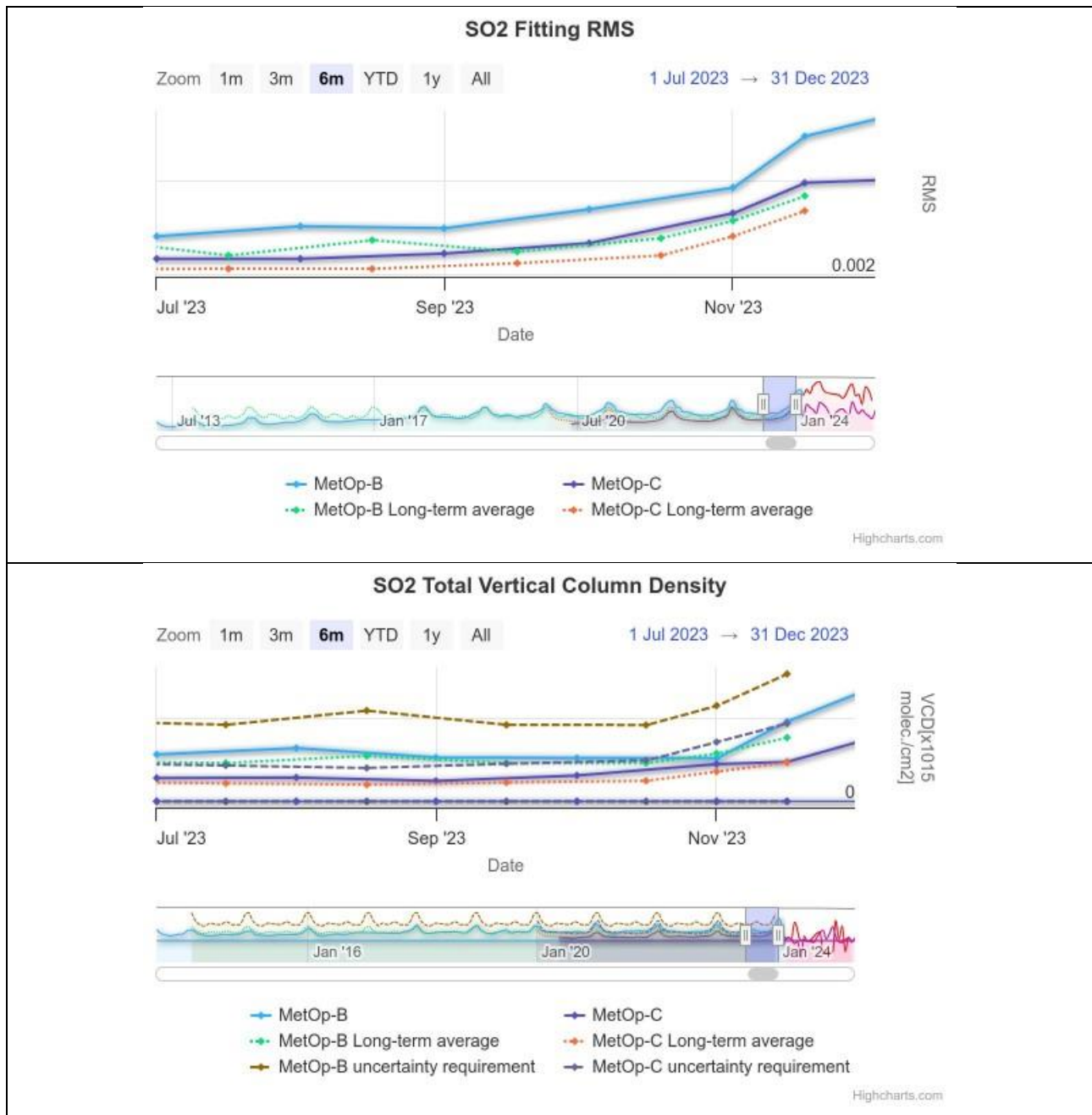
Figure 7.19. The behaviour of the GDP4.8 GOME-2B [blue curve] and GOME-2C [black curve] 1 km plume height SO 2 products between 01/07/2023 and 31/12/2023 over the North China Plane. Upper panel, the SO 2 fitting RMS is shown and in the bottom panel, the total vertical SO 2 column. The equivalent long-term average is also provided [see insert legend].
