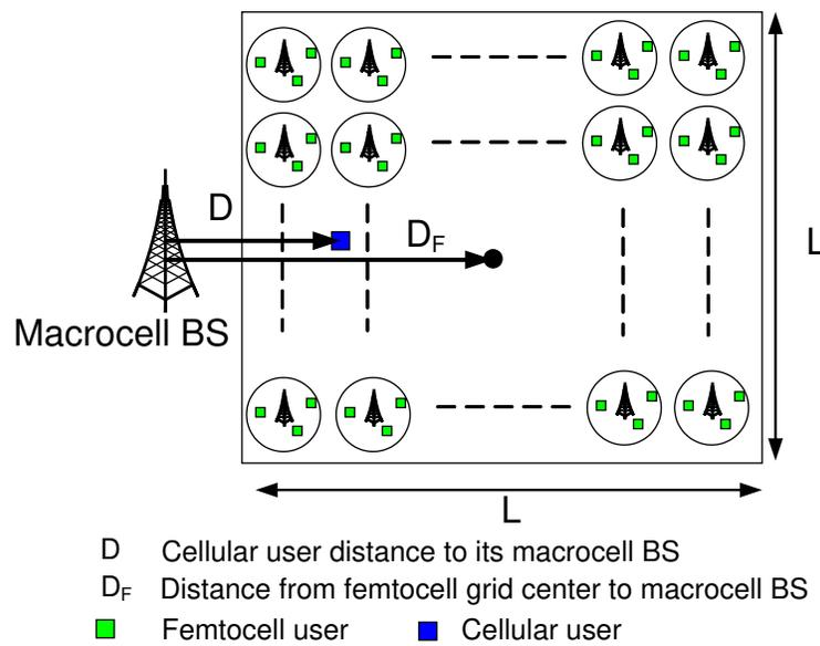
Fig. 2. Single transmitting cellular user transmitting in same spectrum with an underlaid grid of femtocells.
