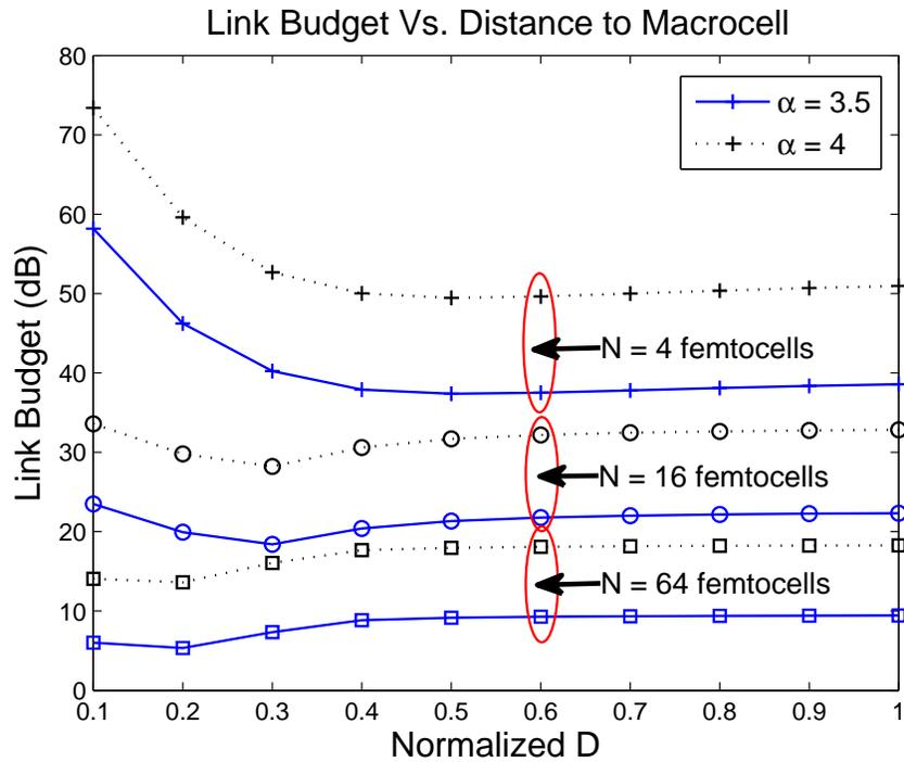
(a) Link budget for a square femtocell grid configuration.
