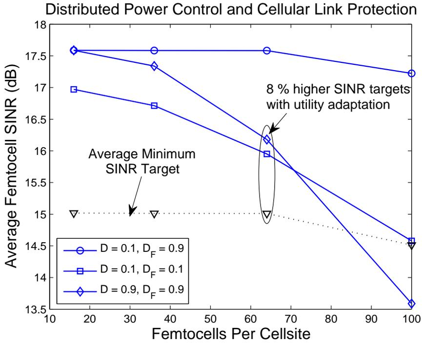
Fig. 6. Mean femtocell SINR targets with distributed power control and cellular link quality protection.
