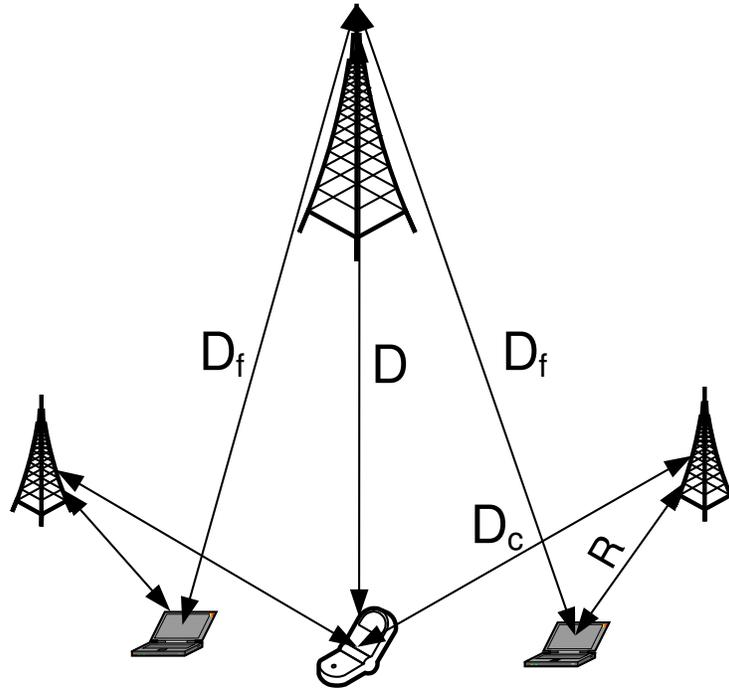
Fig. 1. Simple example with  $N = 2$  femtocells for determining how link budgets vary with the normalized interference distance  $D_f D_c / R_f D$ .
