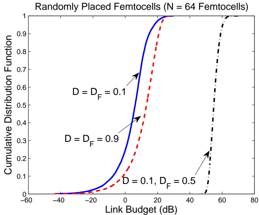
(b) Cumulative distribution function of the link budget  $10 \log_{10}(1/\mathbf{q}_c^T \mathbf{q}_f)$  with randomly located femtocells.Fig. 4. Link budget  $10 \log_{10}(1/\mathbf{q}_c^T \mathbf{q}_f)$  considering a square femtocell grid and randomly placed femtocells.
