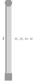
Fig. 1. Protograph of (\alpha, d = 5) LDLC. The circle and rectangle nodes represent variable and check nodes, respectively. Black line denotes a edge labeled 1 and gray lines denote edges labeled w .
