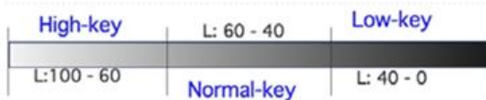
Fig 6. The borders in the L*-scale (Lightness) for high-key, normal-key and low-key images.
