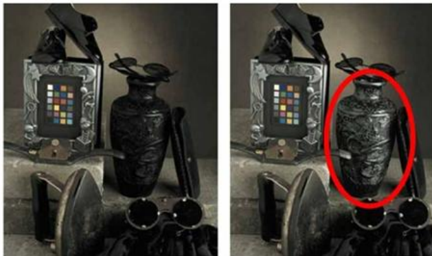
Fig 9. A comparison between low-key images after printing. The image to the left was separated with the standard test chart and the image to the right with the image-adapted test chart.
