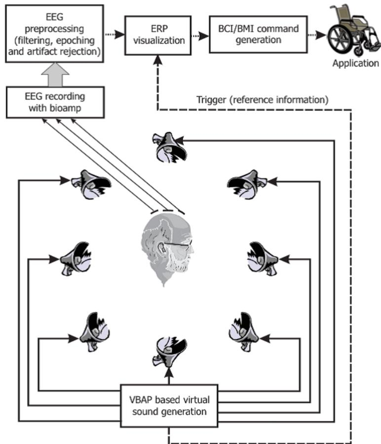
**Figure 1.** Schematic drawing of the proposed auditory BCI system. The subject in the center is surrounded by horizontally distributed loudspeakers. EEG signals are processed by the BCI processing stages in synchrony with presented spatial auditory stimuli.
