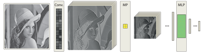
Fig. 1. A schematic representation of an MPCNN. Raw input pixel values are processed by a number of interleaved Convolutional and MaxPooling layers, which are trained to extract meaningful features. Several Fully-Connected layers follow, which produce the final classification.
