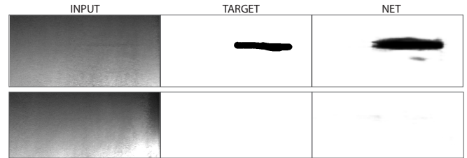
Fig. 5. A typical steel defect example. Segmentation is almost perfect, illustrating the power of the proposed approach for industrial applications.
