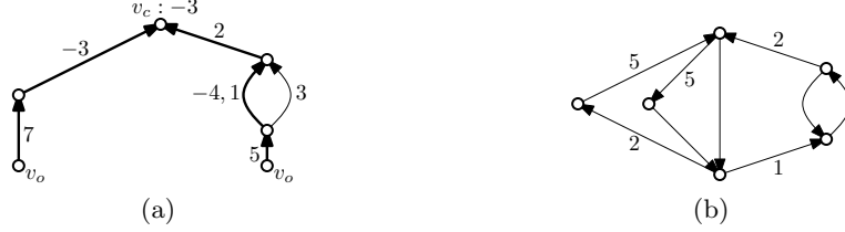
Figure 7: (a) The directed fat tree T' for the residual network of the flow from Figure 6 after we remove all the arcs and vertices which are not on a directed path from a copy of v_o to v_c . The label of each arc is its cost and its capacity, if it is finite (there is only a single arc with finite capacity in this example). There are two copies of v_o in T' . The initial tree \hat{T} is bold . The cost of the minimum cost residual path from the right-hand side copy of v_o to v_c is 5 + (-4) + 2 = 3 . We first send 1 unit of flow along this path, and saturate one of its arcs. After we replace the saturated arc of cost -4 with an arc of cost 3, the minimum cost path from a copy of v_o to v_c is now from the left-hand side copy of v_o . We send 2 units of flow along this path. (b) The final solution, an optimal flow for the network from Figure 5. The label of each arc is the amount of flow assigned to it.
