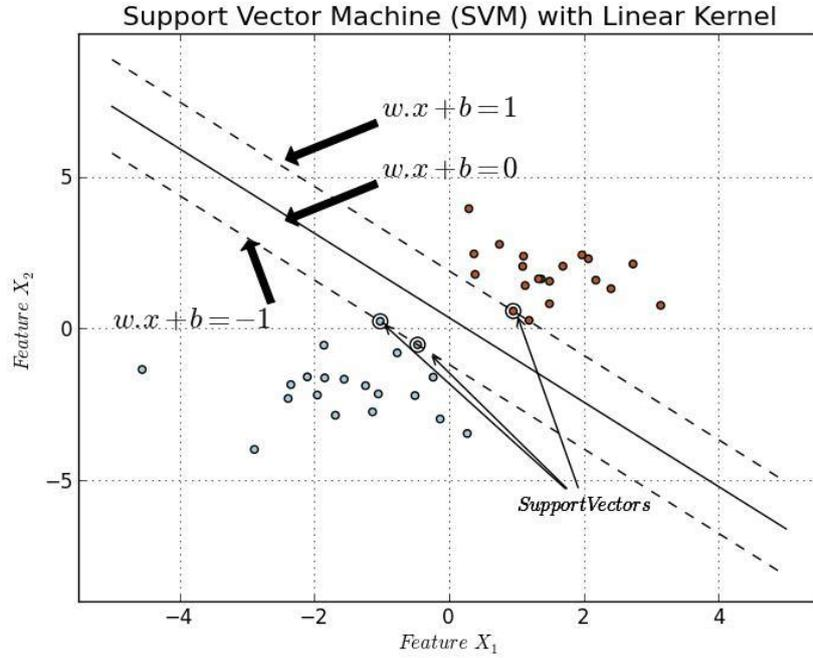
**Figure 1** Classification of an SVM with Maximum-margin hyper plane trained with samples from two classes.
