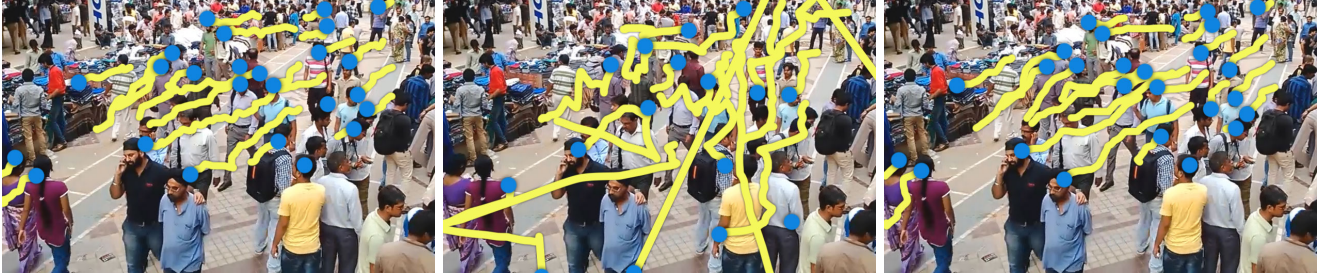
Fig. 2: Performance comparison of our approach with other algorithms on a crowded scene.: (a) Online Boosting [8](11 fps); (b) MeanShift algorithm [9] (33 fps); (c) Our Approach MLPF-RVO (28 fps). Overall, the accuracy of our approach is comparable to Online Boosting and the performance is a little slower than the MeanShift algorithm (Dataset - NPLACE-2)
