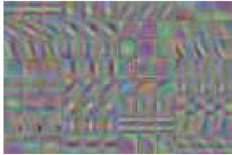
Figure 5. The learned filters of the first level convolutional layers of the multi-scale deep ranking model.
