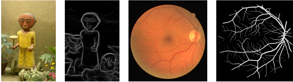
Figure 1: N^4 -Fields can be applied to a range of complex image processing tasks, such as natural edge detection (left) or vessel segmentation (right). The proposed architecture combines the convolutional neural networks with the nearest neighbor search and is generic. E.g. it achieves state-of-the-art performance on standard benchmarks for these two rather different applications with very little customization or parameter tuning.
