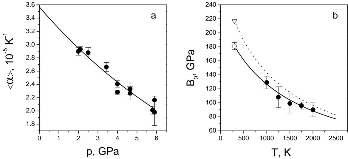
**Figure 3.** Experimental data on (a) pressure dependence of the mean high-temperature coefficient of thermal expansion of  $\text{B}_6\text{O}$  (solid line shows the exponential fit) and (b) temperature dependence of the bulk modulus of  $\text{B}_6\text{O}$  (solid line corresponds to the theoretical line with  $B_0 = 181 \text{ GPa}$ , while dotted line, to  $B_0 = 217 \text{ GPa}$  at 300 K). Solid symbols represent our results, open symbols are literature data [22].
