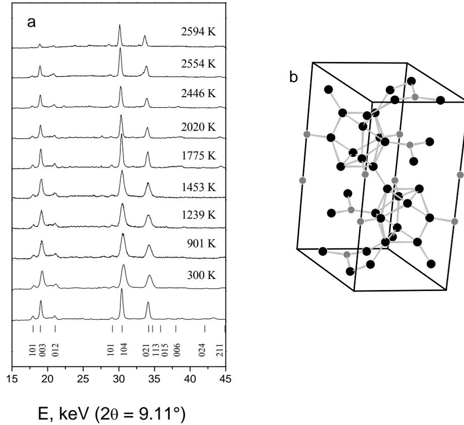
**Figure 1.** (a) Energy-dispersive diffraction patterns of  $B_6O$  taken *in situ* at 4.3 GPa upon heating to 2600 K (the bottom pattern is taken at ambient conditions). (b) Crystal structure of  $B_6O$ . Black and grey balls represent boron and oxygen atoms, respectively.
