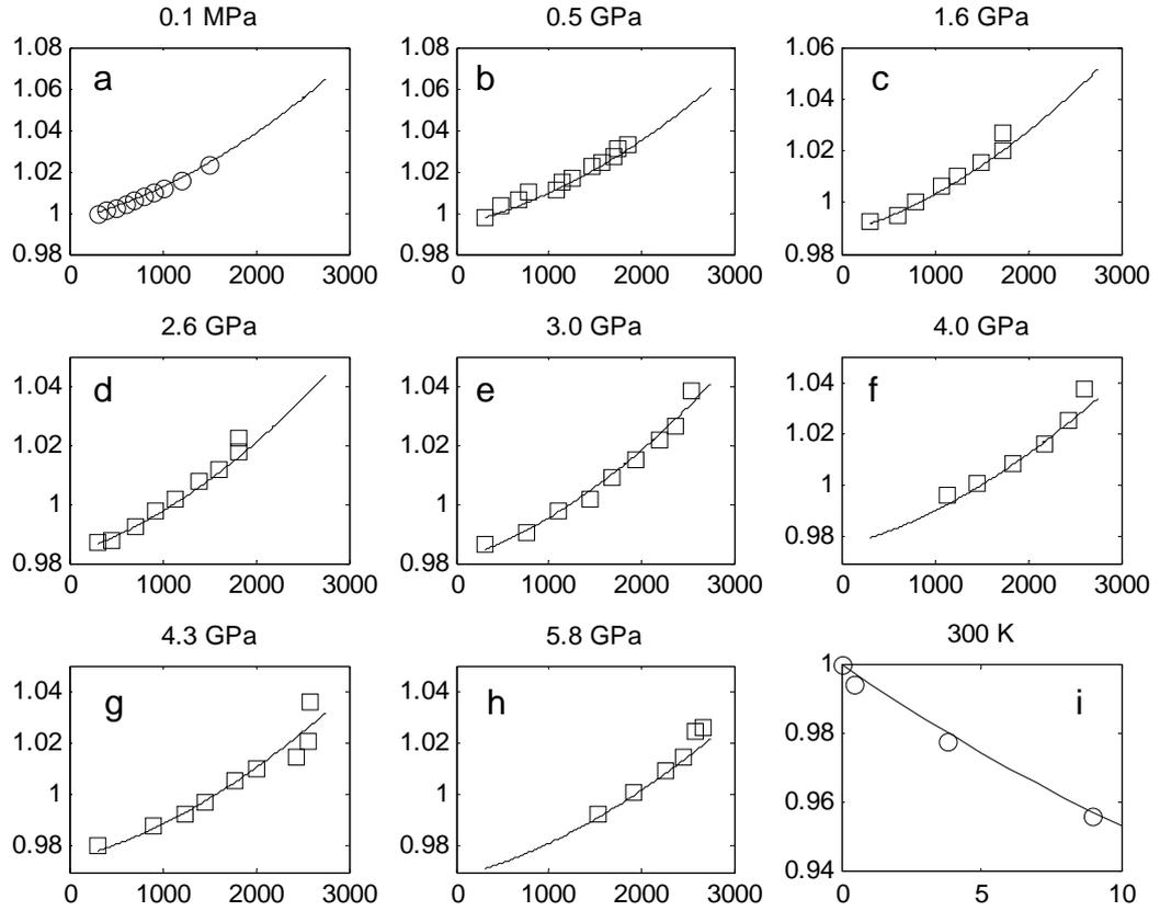
**Figure 2.** (a - h) Temperature dependence of relative volume  $V/V_0$  of  $B_6O$  ( $V_0$  taken at 300 K and ambient pressure). The plot coordinates are  $x - T$  (K) and  $y - V/V_0$ . (i) Pressure dependence of relative volume  $V/V_0$  of  $B_6O$  at 300 K. The plot coordinates are  $x - p$  (GPa) and  $y - V/V_0$ .
