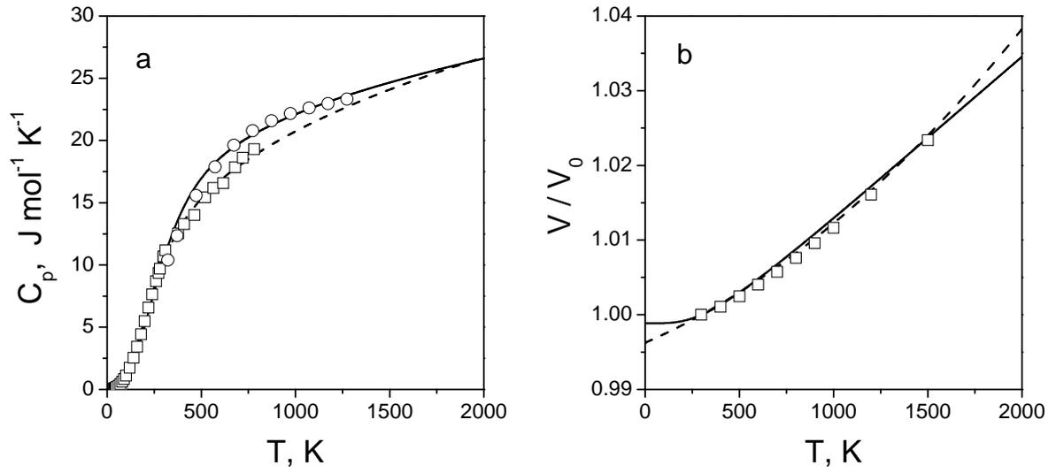
**Figure 4.** Experimental data on (a) heat capacity  $c_p$  of B<sub>6</sub>O as a function of temperature (squares from [23], circles from [26], lines show the results of fitting to Eq. 1); and (b) thermal expansion of B<sub>6</sub>O at 0.1 MPa (squares are experimental data [41], dashed curve corresponds to the square-polynomial fitting (Eq. 6), while solid one – to the numerical solution of Eq. 17 with Grüneisen coefficient  $\gamma = 0.85$ ).
