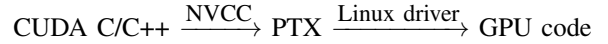
Figure 2: Program representations and compilation steps in the NVIDIA CUDA C/C++ development chain. Our compute kernels are implemented directly with the PTX programming language.
