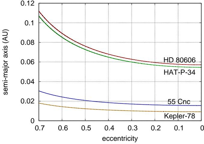
**Fig. 7.** Evolution of the semi-major axis as a function of the eccentricity for different systems and  $\tau$  values. The dotted lines correspond to the theoretical prediction given by expression (83). Solid lines correspond to the orbital evolution obtained using numerical simulations with different  $\tau$  values. For each system, the simulations exactly match the theoretical prediction.
