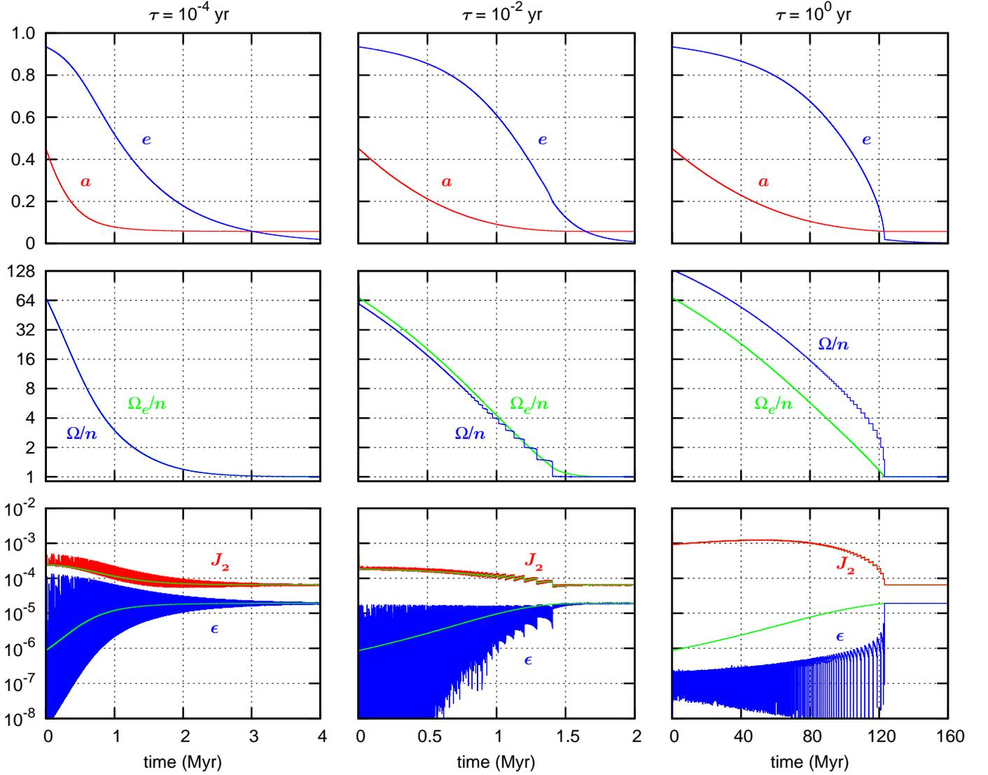
**Fig. 6.** Evolution of HD 80606 b with time for different  $\tau$  values. We plot the semi-major axis (in AU) and the eccentricity (*top*), the ratio between the planet rotation rate and the orbital mean motion (*middle*), and the planet  $J_2$  and  $\epsilon$  (*bottom*). The green line gives the *pseudo-synchronization* equilibrium (Eq. 60) (*middle*), and the average equilibrium values for  $J_2$  and  $\epsilon$ , respectively (Eqs. 85 and 86) (*bottom*).
