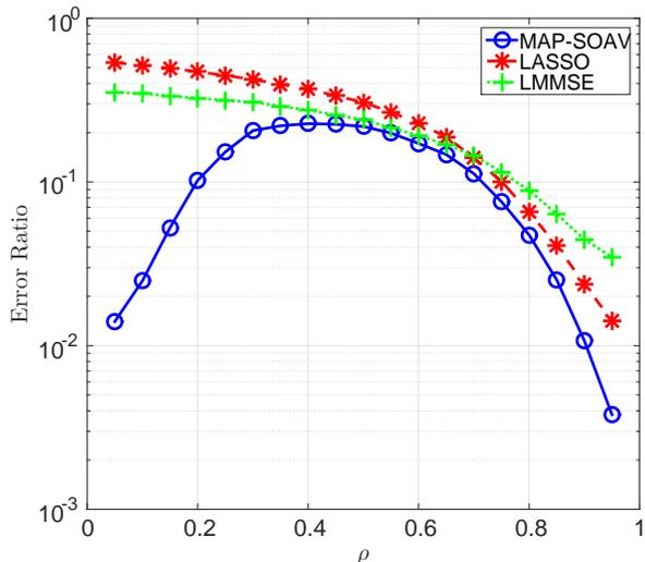
Fig. 7. The non-active rate  $\rho$  vs Error Ratio. The user number  $N$  is 100, the measurement number  $M$  is 70,  $\sigma_w^2$  is 0.0226, and  $S$  is generated by normal Gaussian distribution. (a) The solid line corresponds to MAP-SOAV estimation. (b) The broken line corresponds to LASSO estimation. (c) The dotted line corresponds to LMMSE estimation.
