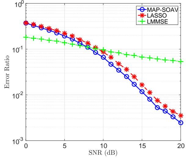
Fig. 5. SNR vs Error Ratio when the non-active rate  $\rho$  is 0.8. The user number  $N$  is 100, the measurement number  $M$  is 70, and  $S$  is generated by normal Gaussian distribution. (a) The solid line corresponds to MAP-SOAV estimation. (b) The broken line corresponds to LASSO estimation. (c) The dotted line corresponds to LMMSE estimation.
