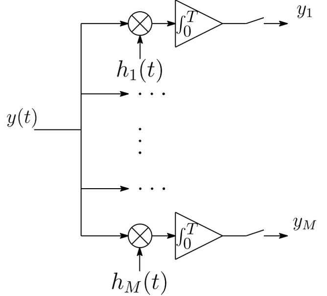
Fig. 2. Filter bank at the receiver.
