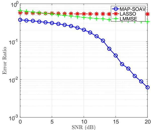
Fig. 6. SNR vs Error Ratio when the non-active rate  $\rho$  is 0.05. The user number  $N$  is 100, the measurement number  $M$  is 70, and  $S$  is generated by normal Gaussian distribution. (a) The solid line corresponds to MAP-SOAV estimation. (b) The broken line corresponds to LASSO estimation. (c) The dotted line corresponds to LMMSE estimation.
