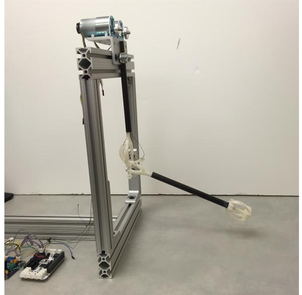
Fig. 9. The physical prototype of our tensegrity elbow. Compression elements are composed of 3D-printed Poly-lactic Acid (PLA) and tension elements are composed of spectra braided fishing line. This model is actively controlled by motors seen mounted off of the robot and onto the chassis.
