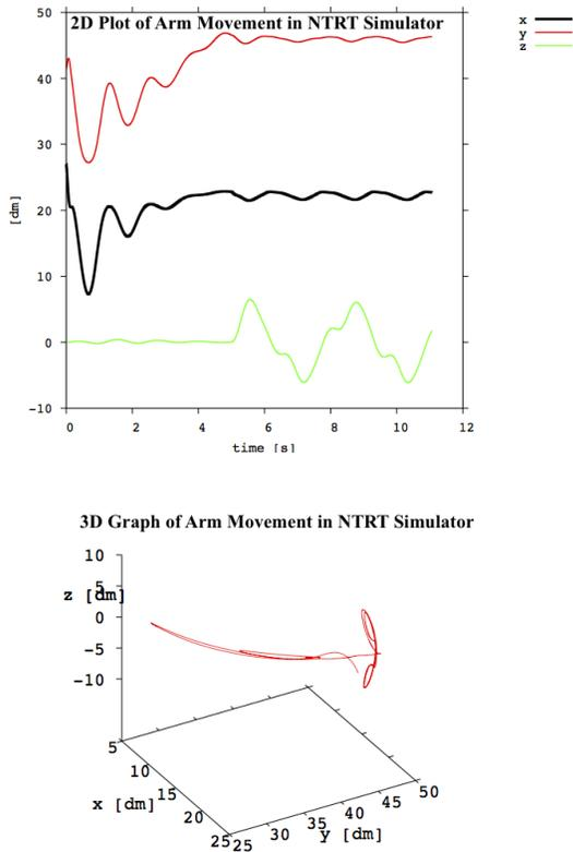
Fig. 4. The movement of the end-effector of our simulated tensegrity arm with respect to time. The plotted path illustrates the arm as it demonstrates pitch motion and then yaw motion.
