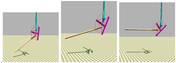
Fig. 5. A simulated tensegrity elbow demonstrating pitch movement. Two cables, mimicking the bicep and tricep in function, act as the antagonistic pair responsible for generating this movement.
