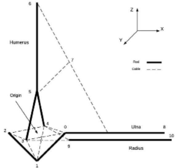
Fig. 2. The design for the first passive structure simulated. This was based upon Scarr's passive tensegrity elbow [7]
