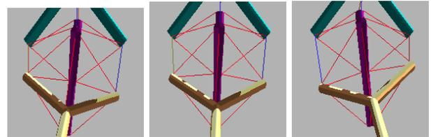
Fig. 6. A simulated tensegrity elbow demonstrating yaw movement. Unlike pitch movement, yaw movement is not generated in the elbow, but instead in the shoulder in an anatomically accurate human arm.
