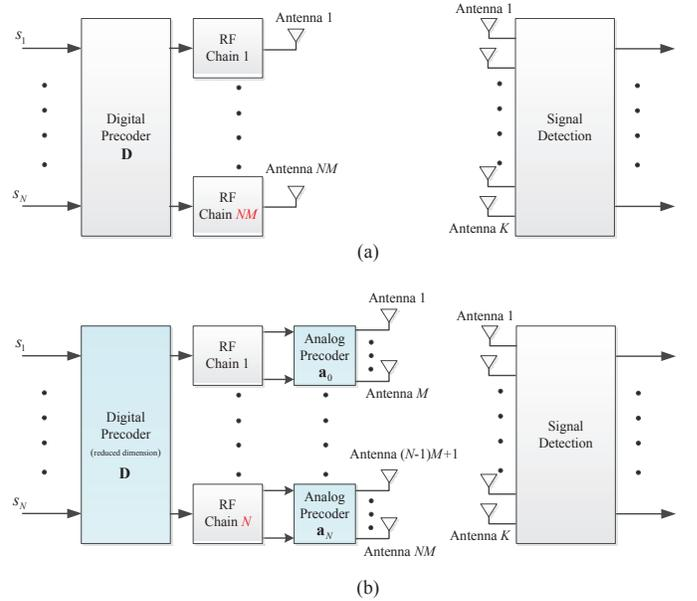
Fig. 1. Architecture comparison: (a) Fully digital precoding in conventional massive MIMO; (b) Hybrid analog/digital precoding in mmWave massive MIMO with sub-array structure.
