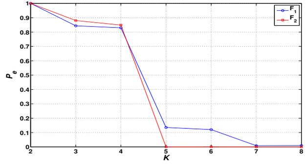
Fig. 3: Probability of  $\|\mathbf{s} - \hat{\mathbf{s}}\| > 0$  as a function of collision size  $K$  for ETF structure.
