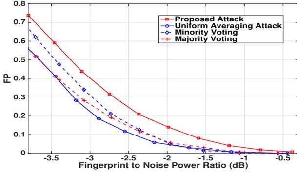
Fig. 10: Comparison of the false positive (FP) probabilities of different attacks against the Tardos code with parameter  $(k, \epsilon) = (5, 0.1)$ .
