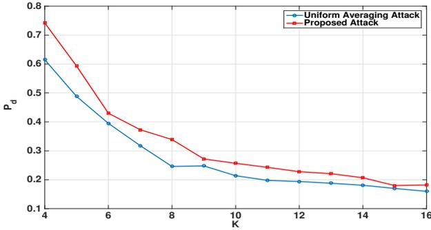
Fig. 6: A comparison of probability of detecting at least one colluder for our proposed attack vs. uniform linear averaging attack as a function of number of colluders for random Gaussian fingerprints  $((N, M) = (100, 250))$ .
