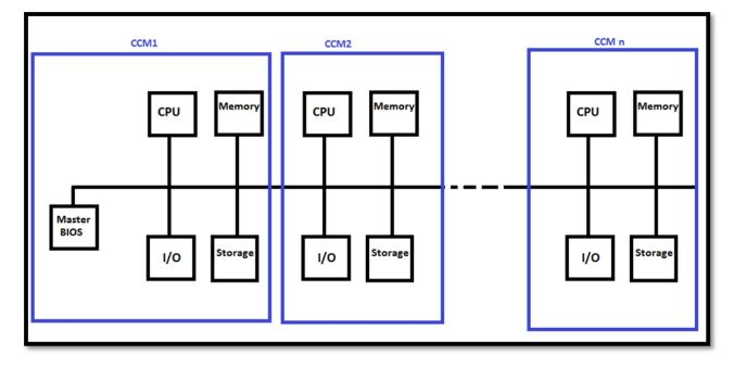
FIGURE 6 BLOCK DIAGRAM OF CCM POOL
