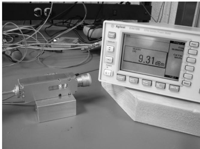
Fig. 12. Photograph of module A delivering a 9.3 dBm CW tone at 90 GHz, with a power meter for comparison.
