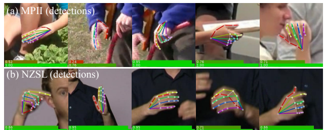
Figure 8: Detections using model “Mix 3” on test images. To show a representative sample, we pick the first 5 images from the test sets of (a) MPII, and (b) NZSL. Each image’s PCK at \sigma = 0.1 and \sigma = 0.2 (across the 21 keypoints) is shown as a pair of bars at the bottom of the image, colored from red (0) to green (1).
