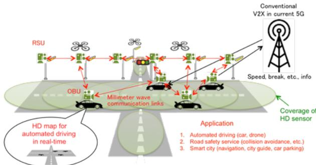
Figure 23: mmWave based V2V/V2X to exchange HD maps
