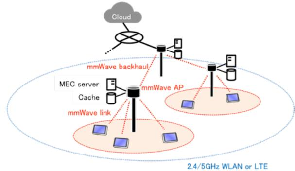
Figure 6: System architecture example composed of mmWave access and mobile edge computing
