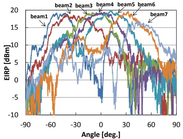
Figure 8: Measured output power with different beams (at 58.32 GHz)
