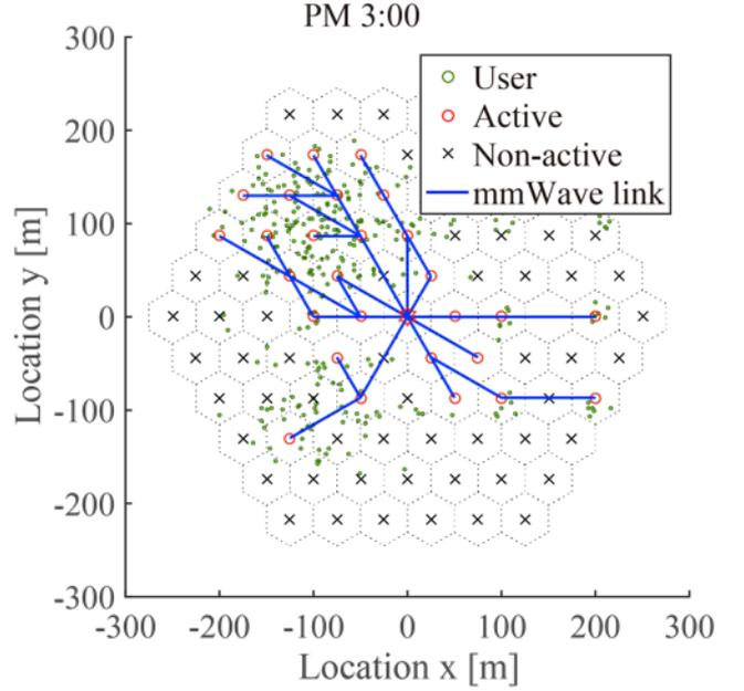
(b) Formed mmWave mesh network at PM 3:00.
