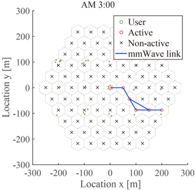
(a) Formed mmWave mesh network at AM 3:00.
