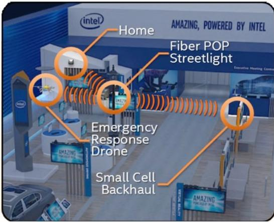
Figure 21 mmWave mesh node to provide three different backhaul links exhibited in MWC2017
