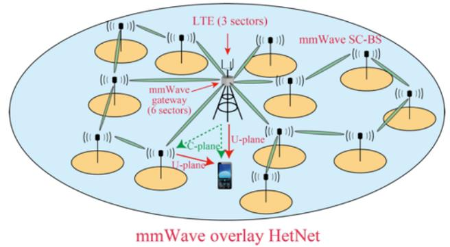
Figure 14: mmWave mesh network overlaid on a macro cell
