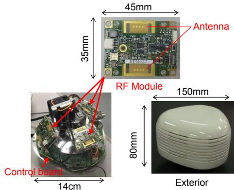
Figure 7: Prototype of 60 GHz IEEE802.11ad / WiGig access point
