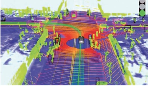
Figure 22: HD map measured by LiDAR as a high-resolution point cloud [60]
