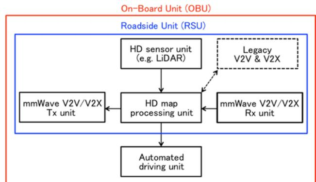
Figure 24: RSU and OBU composed of mmWave and MEC
