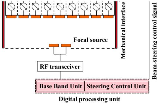
**Figure 4** Schematic view of the backhauling base station with electronically steerable transmit array
