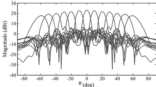
**Figure 5** Simulated analogue beamforming capability of the linearly-polarized transmit array developed in 5G CHAMPION at 28 GHz (E-plane gain radiation pattern).
