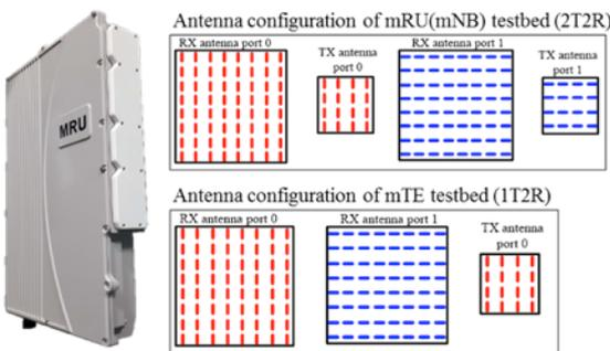
Figure 2 Antenna configurations of South Korean 28 GHz backhaul testbed.
