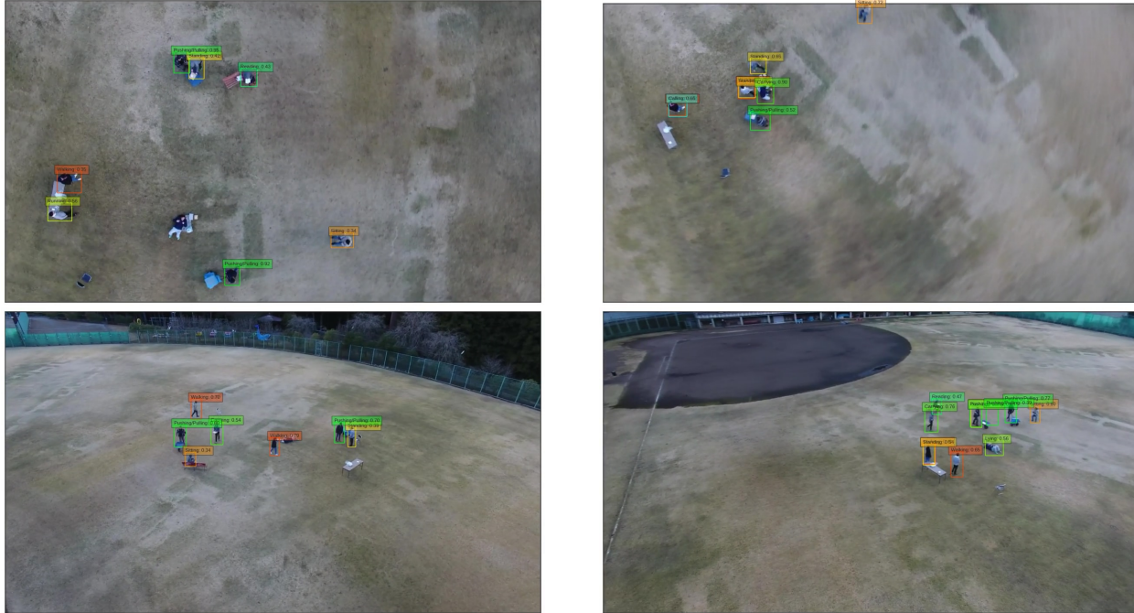
Figure 6: Sample detections of SSD 960x540 model for action detection. Detections with confidence score higher than 0.3 are shown. Each color corresponds to an action category. Frames from Okutama-Action test set.
