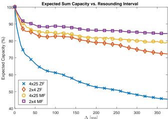
Fig. 4. Expected sum-rate for ZF and MF versus channel resounding interval  $\Delta$  across the full 30 s mobile scenario
