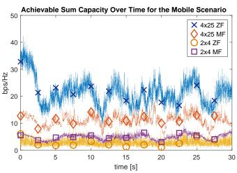
Fig. 2. Achievable sum-rate over time for the full mobile scenario using ZF and MF for 100 and 8 BS antennas serving 4 dual-antenna USRPs clients (8 streams). Average SNR fixed to 30 dB
