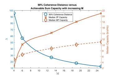
Fig. 3. Terminal distance moved in wavelengths for 10% spatial decorrelation versus median achievable sum-rate. M represents the number of elements in the azimuth for the  $4 \times M$  array.
