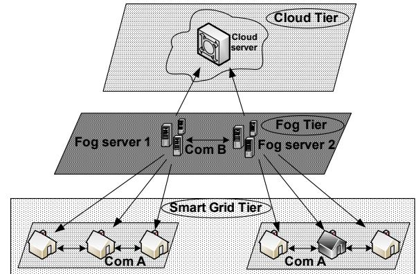
Fig. 5 Hierachal communication structure of the Fog computing.
