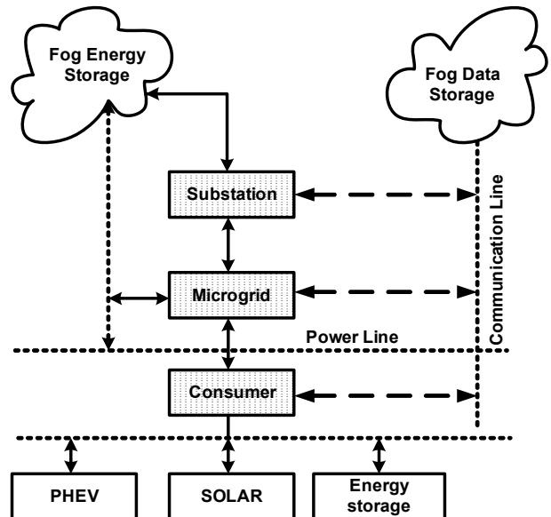
Fig. 7 Microgrid concept using Fog computing.
