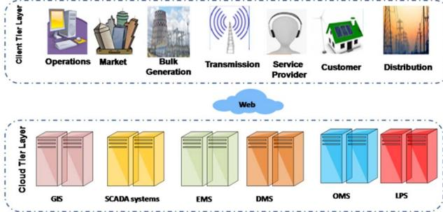
Fig. 3 Cloud Computing Framework of smart grid system.
