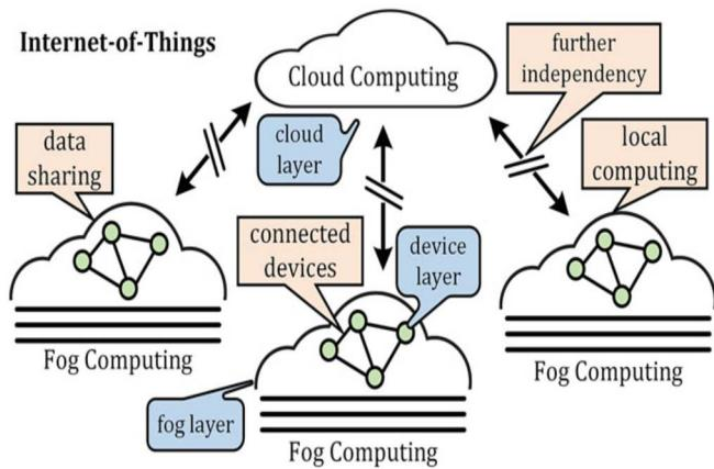
Fig. 8 Implementing Fog computing as an intermediary layer to cloud computing in Internet-of-Things (IoT) platform.
