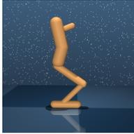
**Hopper (14, 4, 15):** The planar one-legged hopper introduced in (Lillicrap et al., 2015), initialised in a random configuration. In the **stand** task it is rewarded for bringing its torso to a minimal height. In the **hop** task it is rewarded for torso height and forward velocity.
