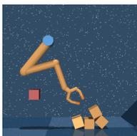
**Stacker (6k+16, 5, 11k+26):** Stack  $k$  boxes. Reward is given when a box is at the target and the gripper is away from the target, making stacking necessary. The height of the target is sampled uniformly from  $\{1, \dots, k\}$ .
