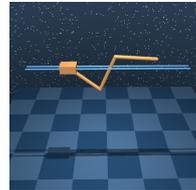
**Cart-k-pole (2k+2, 1, 3k+2):** The cart-pole domain allows to procedurally adding more poles, connected serially. Two non-benchmarking tasks, **two\_poles** and **three\_poles** are available.
