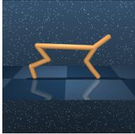
**Cheetah (18, 6, 17):** A running planar biped based on (Wawrzyński, 2009). The reward  $r$  is linearly proportional to the forward velocity  $v$  up to a maximum of  $10_{\text{m/s}}$  i.e.  $r(v) = \max(0, \min(v/10, 1))$ .
