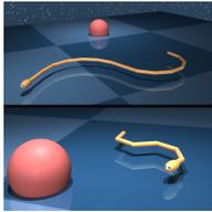
**Swimmer ( $2k+4$ ,  $k-1$ ,  $4k+1$ ):** This procedurally generated  $k$ -link planar swimmer is based on (Coulom, 2002) but using MuJoCo’s high-Reynolds fluid drag model. A reward of 1 is provided when the nose is inside the target and decreases smoothly with distance like a Lorentzian. The two instantiations provided in the **benchmarking** set are the 6-link and 15-link swimmers.
