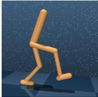
**Walker (18, 6, 24):** An improved planar walker based on the one introduced in (Lillicrap et al., 2015). In the **stand** task reward is a combination of terms encouraging an upright torso and some minimal torso height. The **walk** and **run** tasks include a component encouraging forward velocity.
