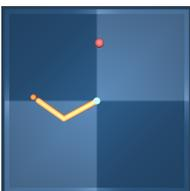
**Reacher (4, 2, 7):** The simple two-link planar reacher with a randomised target location. The reward is one when the end effector penetrates the target sphere. In the **easy** task the target sphere is bigger than on the **hard** task (shown on the left).
