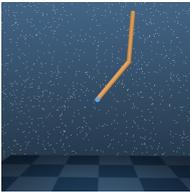
**Acrobot (4, 1, 6):** The underactuated double pendulum, torque applied to the second joint. The goal is to swing up and balance. Despite being low-dimensional, this is not an easy control problem. The physical model conforms to (Coulom, 2002) rather than the earlier (Spong, 1995). Both **swingup** and **swingup\_sparse** tasks with smooth and sparse rewards, respectively.
