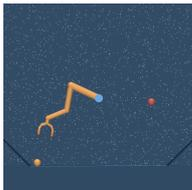
**Manipulator (22, 5, 37):** A planar manipulator is rewarded for bringing an object to a target location. In order to assist with exploration, in %10 of episodes the object is initialised in the gripper or at the target. Four **manipulator** tasks: **{bring,insert}\_{ball,peg}** of which only **bring\_ball** is in the **benchmarking** set. The other three are shown below.
