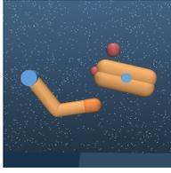
**Finger (6, 2, 12):** A 3-DoF toy manipulation problem based on (Tassa and Todorov, 2010). A planar ‘finger’ is required to rotate a body on an unactuated hinge. In the **turn\_easy** and **turn\_hard** tasks, the tip of the free body must overlap with a target (the target is smaller for the **turn\_hard** task). In the **spin** task, the body must be continually rotated.
