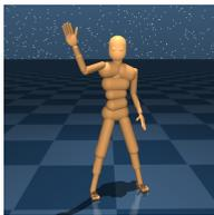
**Humanoid\_CMU (124, 56, 137):** A humanoid body with 56 joints, adapted from (Merel et al., 2017) and based on the ASF model of subject #8 in the **CMU Motion Capture Database**. This domain has the same **stand**, **walk** and **run** tasks as the simpler humanoid. We include tools for parsing and playback of the CMU MoCap data, see below.
