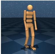
**Humanoid (54, 21, 67):** A simplified humanoid with 21 joints, based on the model in (Tassa et al., 2012). Three tasks: **stand**, **walk** and **run** are differentiated by the desired horizontal speed of 0, 1 and  $10_{m/s}$ , respectively. Observations are in an egocentric frame and many movement styles are possible solutions e.g. running backwards or sideways. This facilitates exploration of local optima.
