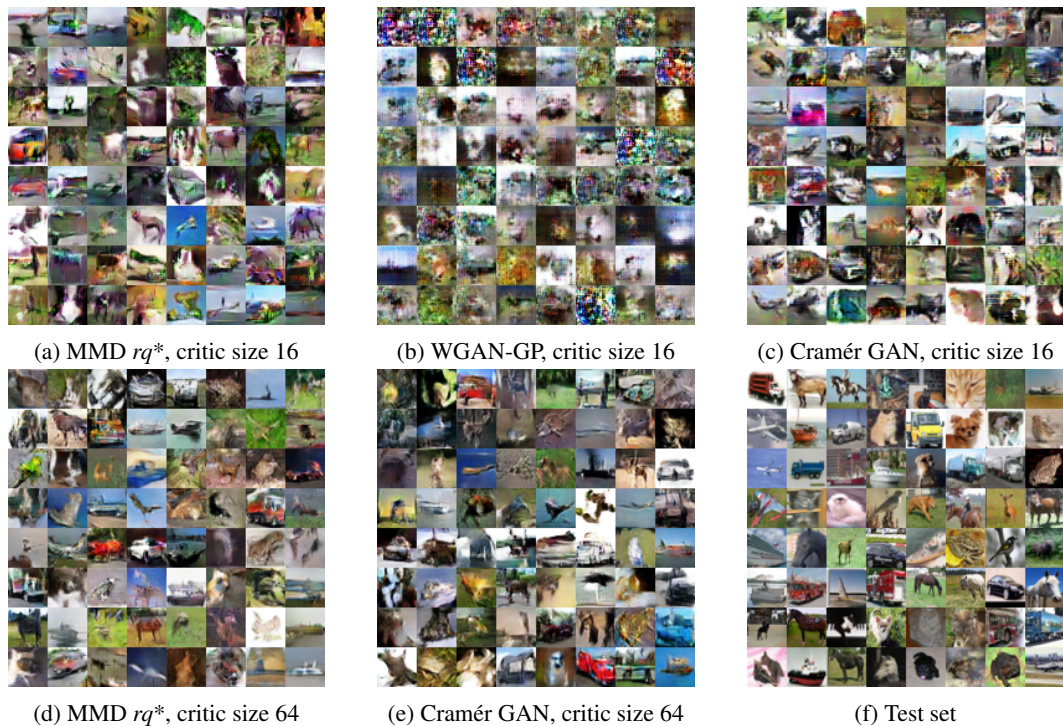
Figure 13: Comparison of samples from various models, as well as true samples from the test set. WGAN-GP samples with critic size 16 are quite bad. Cramer GAN samples with critic size 16 are more appealing to the eye, but seem to have pixel-level issues. Large-critic Cramer and MMD rq^* GAN are of similar quality.
