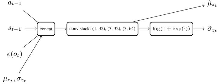
Figure 13. Posterior module for computing mean  $\hat{\mu}_{z_t}$  and diagonal variance  $\hat{\sigma}_{z_t}$  of the normal distribution  $q(z_t | s_{t-1}, a_{t-1}, o_t)$ . The posterior gets as additional inputs the prior statistics  $\mu_{z_t}, \sigma_{z_t}$ .
