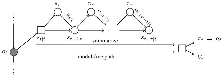
Figure 2. The architecture of the Imagination-Augmented Agent, which computes its policy  $\pi_t$  and value function  $V_t$ , by combining information from a model-free path with information from Monte-Carlo rollouts of its environment model.
