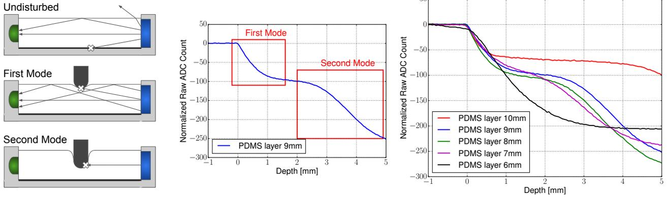
Fig. 6. **Left and middle:** interaction modes. The first mode of detection happens upon light contact and manifests as a sudden drop in the signal. The second mode is activated with a heavier contact, in this particular case after a depth of approximately 2mm. **Right:** we investigated this behavior for different heights of the PDMS layer, in order to select one for which these two modes are contiguous.
