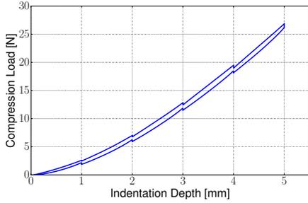
Fig. 3. Load vs indentation depth for a 1:20 ratio of curing agent to PDMS, measured by advancing or retracting the probe in 1mm steps with 10s pauses using a 6mm diameter hemispherical tip.
