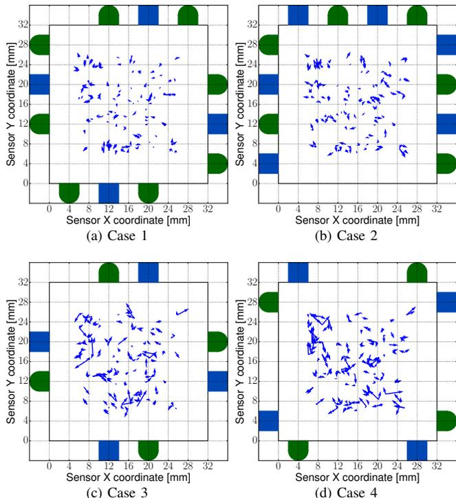
Fig. 10. Localization error at 2mm indentation depth for cases where sensing terminals have been removed from our base configuration. Green semicircles (diodes) and blue squares (LEDs) indicate the terminals present in each case.
