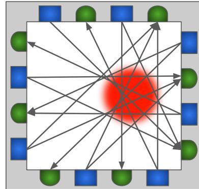
Fig. 1. Spatially Overlapping Signals. Arrows represent the spatial receptive field of a given pair of sensing terminals. A single contact affects signals extracted from multiple pairs whose receptive fields overlap on the contact location.
