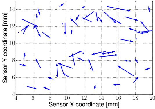
Fig. 4. Magnitude and direction of localization errors for resistive sensor. Each arrow represents one test indentation: the base of the arrow is at the ground truth location while the tip is at the predicted location.
