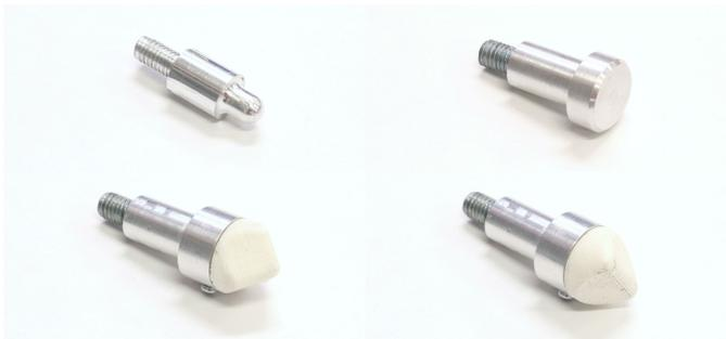
Fig. 12. The four different indenter types used for our classification: hemispherical, flat, corner and edge tips. The edge tip (lower right) was used with orientations of 0, 120 and 240 degrees.
