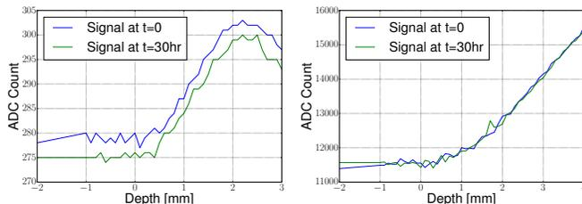
Fig. 11. Signal comparison over time for two versions of our optics-based sensors, with THT components (Left) and SMT components (Right). In each case, we performed 60 consecutive indentations with the 6mm diameter hemispherical tip in a single sensor location, with the indentations spaced 30 minutes apart. Each plot shows the signal from the first and last indentation in the respective set.
