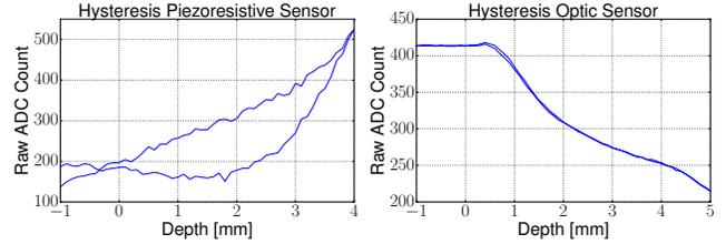
Fig. 5. Hysteresis graph for piezoresistive and optic sensors. Graphs show a single terminal pair response to an indentation up to 4mm and 5mm respectively. A hemispherical indenter was used in both cases.
