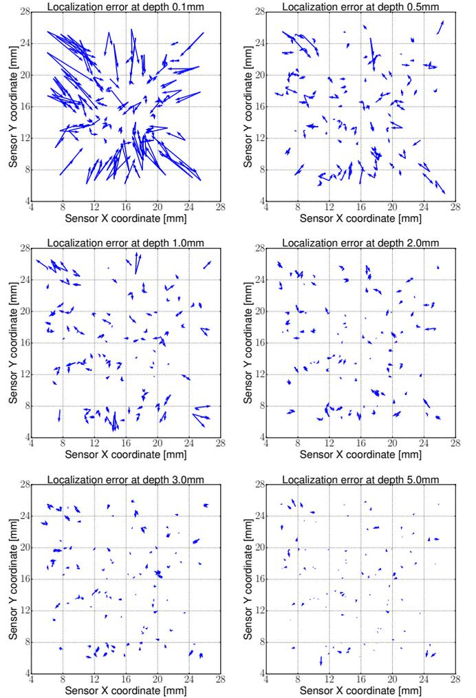
Fig. 9. Localization results for ambient light test dataset. Each arrow represents one indentation in our test set; the base is at the ground truth location while the tip of the arrow shows the predicted location.
