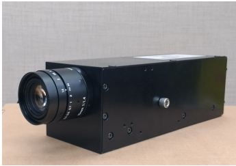
Fig. 1. NH-AIK Hyperspectral camera used for data collection
