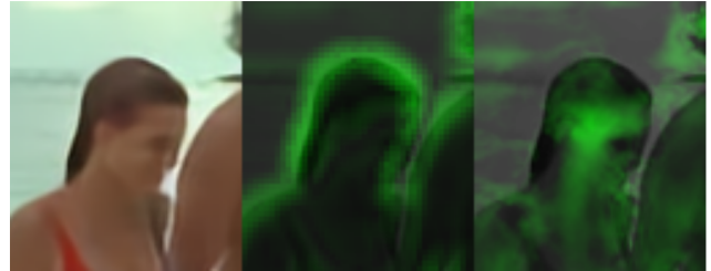
Fig. 1. Perceptual metrics can be trained to respect high-level semantic information such as faces. (a) the distorted image, (b) its perceived distortion under a contrast-based metric and, (c) the same for the proposed perceptual metric, indicating that distortions to a face are more objectionable than distortions to edges. Higher green intensity means higher predicted distortion.
