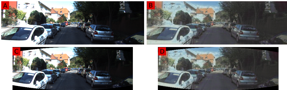
Fig. 2: Output of each step of the adaptation of an image from the KITTI dataset: A: No transformation, B: Style transfer, C: Projection transfer, D: Style and projection
