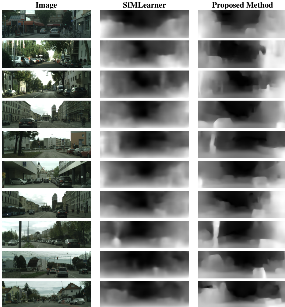
Figure 4. Results of depth estimation compared with SfMLearner on the Cityscapes dataset. Note that the models that were trained only on the KITTI dataset are tested directly on the Cityscapes dataset without any fine-tuning. These images are previously unseen by the networks. (Pictures best viewed in colour.)
