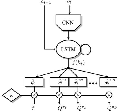
Figure 2. Deep architecture used. Rectangles represent MLPs.
