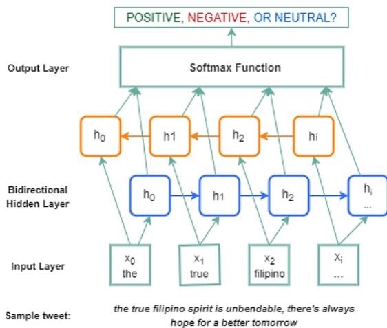
Figure 4. Architecture of bidirectional RNN used in this study
