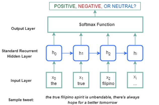
Figure 3. Architecture of standard RNN used in this study
