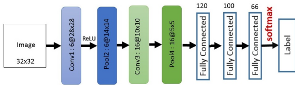
Fig. 8. The original LeNet used for classifying 66 classes.
