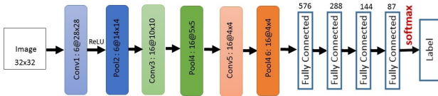
Fig. 9. The modified LeNet for classifying 87 classes
