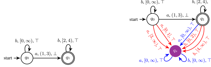
Fig. 1: A DOTA \mathcal{A} on the left and the corresponding COTA \mathbb{A} on the right. The initial location is indicated by ‘start’ and an accepting location is doubly circled.
