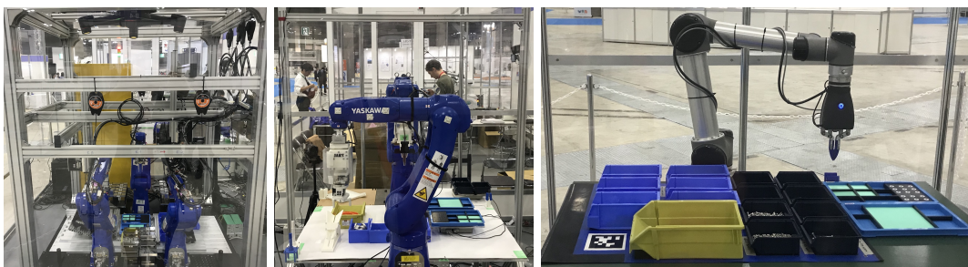
Figure 3. Sample solutions to the kitting task from the teams Robot System Integrators, JAKS, and Robotic Materials (from left to right). The different solutions illustrate the drastically varying use of external sensors and utilities such as tool changers.
