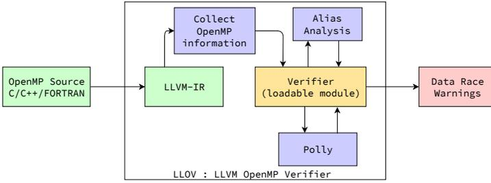
Fig. 1. Flow Diagram of LLVM OpenMP Verifier (LLOV)
