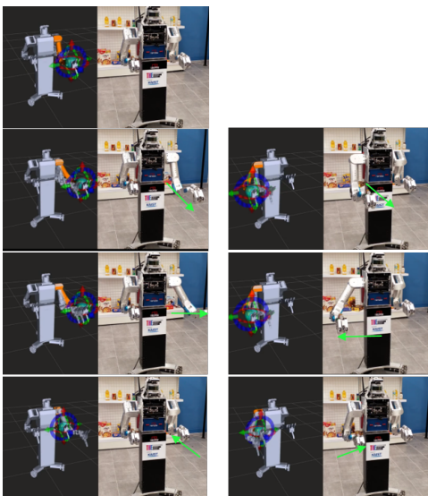
Fig. 11: Timelapse depicting the robot following the requested motion trajectories generated in ROS
