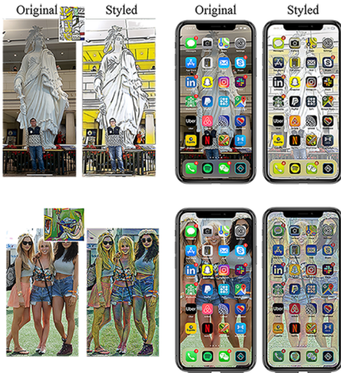
Figure 4: Style transfer applied to the iOS home screen. We show, from left to right, a given style image, a user-supplied photo, a re-styled photo given the style, the original home-screen, and the new theme with re-styled icons and the re-styled photo as a background. Best viewed digitally in full resolution.
