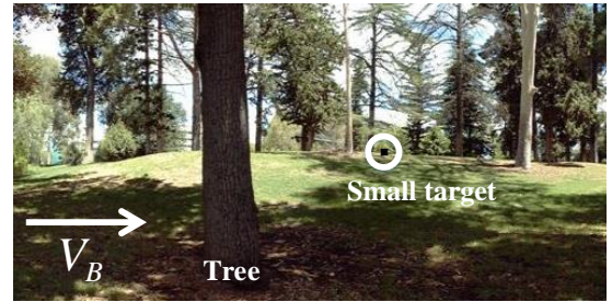
Fig. 8. Input image at time t_0 = 750 ms where a small target (the black block) is moving against the cluttered natural background. The velocity of the small target is set to 250 pixels/s, while that of the background is lower (150 pixels/s). Arrow V_B denotes the motion direction of the background. The tree is considered as a large object moving with the background at the same velocity.
