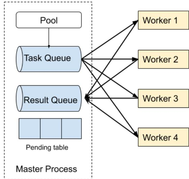
Figure 2: **Task execution failure handling.** Fiber implements task queues, result queues and pending tables. When a task is fetched from the task queue, an entry is added to the pending table. Tasks successfully executed are added to the result queue, while failed tasks are resubmitted to the task queue according to the corresponding entry in the pending table.
