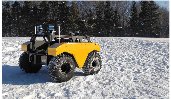
Figure 1: The wheeled skid-steer platform, a Warthog from Clearpath , on a snow-covered testing site. Due to the steering type and the snow on the ground, the robot is very prone to skidding and slippage, making the control and state estimation of this system quite challenging.
