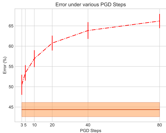
Fig. 1. Mean and standard deviation of the error of the transfer-learned model under different numbers of PGD steps. We fix the step size of PGD to 0.05 in the normalized image space, and use \epsilon = 8/255 . The underlying line shows the mean and standard deviation of the error under Gaussian random perturbation with the same magnitude. All results are based on 4 runs with different random initial perturbations.
